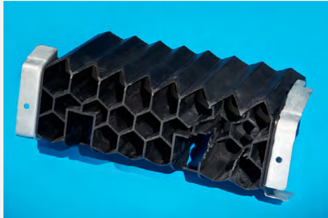
Plastic honeycomb floor rocker reinforcement
