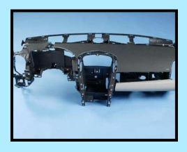
Long-Fiber Reinforced Thermoplastic in Instrument Panels
