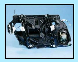
Thermoplastic Door Module and Carrier
