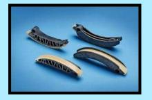
CLTE, plus high knitline strength at the pivot. A separate unfilled nylon 4/6 wear surface is also used. The system provides 30% cost and 20% mass savings vs. previous metal designs, eliminates the need for a hardened-metal wear pin, eliminates 5 machining operations/part, provides tooling savings of \$200,000 USD/year, and is quieter.
